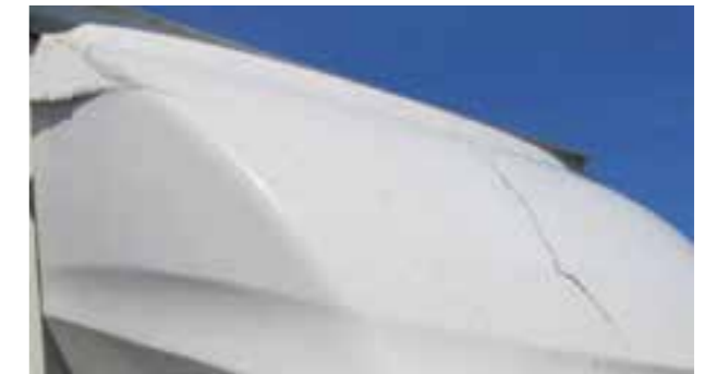
Cabover and deflector: Significant crack, missing part or beyond economic repair
