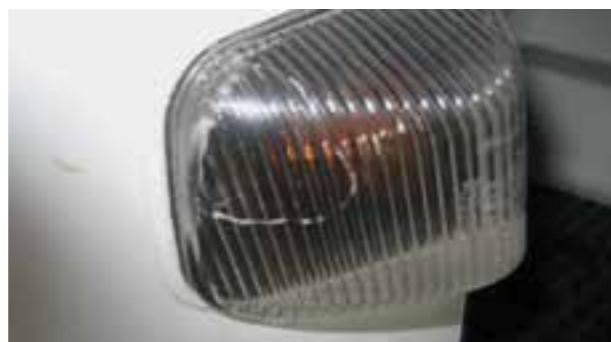
Rear and front lights broken
