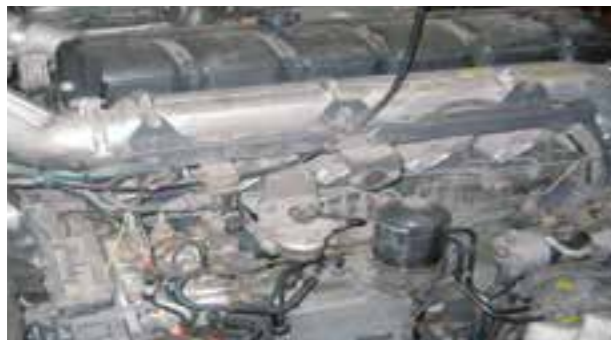
Light traces of oil (no dripping)
