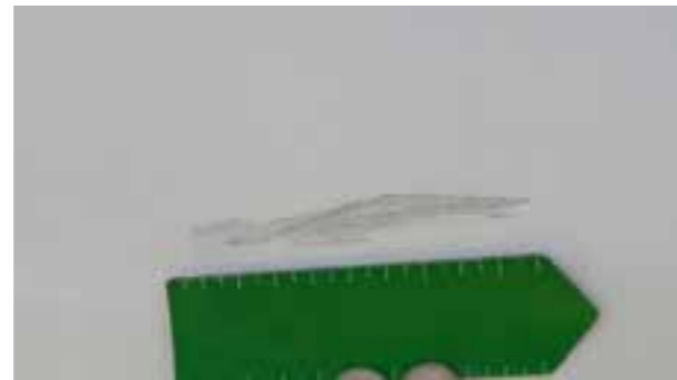
Side panels: Faint scratch with material removal less than 20 cm in length
