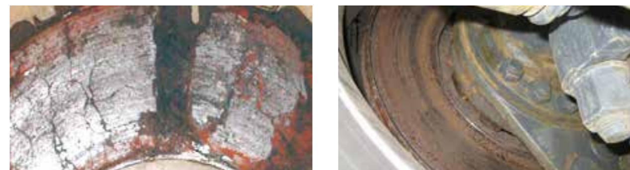
Rusted, ground, worn brake discs
